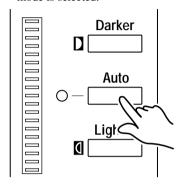
2 Depress the appropriate Exposure Adjustment Button, either LIGHTER or DARKER, to set the desired image density, or exposure, level.
